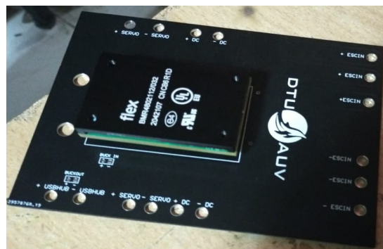
Power distribution board
